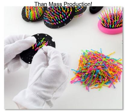
Except for the plastic injection, the rest of the process is carried out 100% by hand, from attaching each tooth one at a time to the final packaging, making our brush a handmade product.
